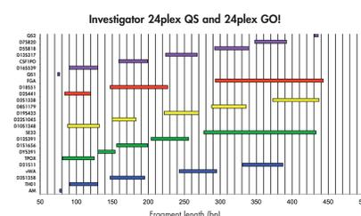
**Marker arrangement.** Marker ranges cover all alleles of the allelic ladder and are displayed according to the dye label used.
