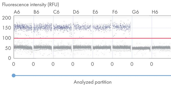
**Figure 4. dPCR Copy Number Assay validation.** 1D scatter plot showing single-well assay validation data of dPCR Copy Number Assay MYC with different human gDNA input amounts (A6–C6: 6 ng/reaction, D6–F6: 4 ng/reaction, G6: NTCs; Green channel for EvaGreen detection).
