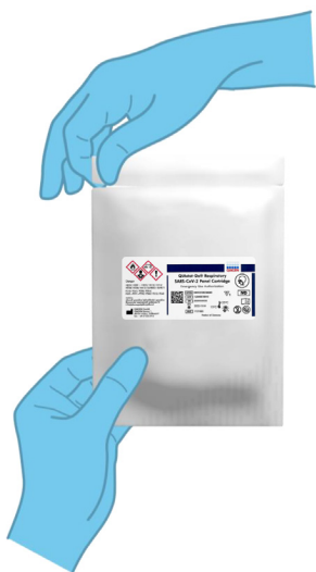
Figura 37. Abrindo o QIAstat-Dx Respiratory SARS-CoV-2 Panel Cartridge.
