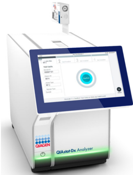
Figura 15. Inserindo o QIAstat-Dx Respiratory SARS-CoV-2 Panel Cartridge no QIAstat-Dx Analyzer 1.0 ou no QIAstat-Dx Analyzer 2.0.
