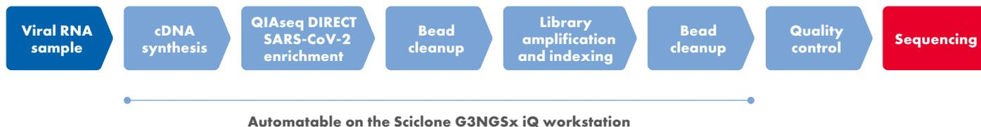
Figure 1. Sample to sequencing workflow showing the automatable library preparation steps.
