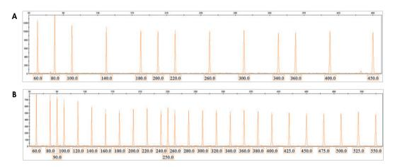
Figure 4. A DNA Size Standard 450 (BTO) with 13 fragments. B DNA Size Standard 24plex (BTO) with 26 fragments.
