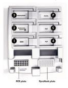
Figure 1. Placement of PCR plate and PyroMark Q24 plate on the vacuum workstation.
