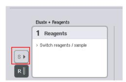
The "Reagents" slot will then switch to a "Sample" slot. This slot will be automatically selected and will be highlighted dark yellow.
