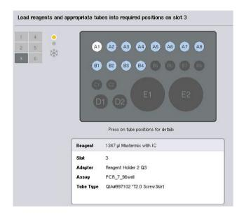
$5. \ \ \text{Press an individual position to view loading information for that particular position}.$
