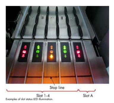
2. Gently slide the tube carrier into the appropriate slot. Insert up to the stop line, and wait until the bar code reader has moved forward.
