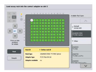
Press an individual position to view information about the sample at that position. You can also use the arrows to select a position. When **Sample** is pressed, the sample ID, sample type, status, and volume are displayed, as well as the assay to which this sample has been assigned.
