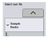
There are 2 types of rack files — **Sample Racks** and **Assay Racks**. **Sample Racks** are standard sample rack files for defining an assay run. In some cases, the assay rack can be used as a sample rack (e.g., for setting up two-step RT-PCR assays). In this case, an **Assay Rack** can be selected.
