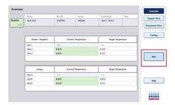
If an inventory scan was performed after pressing the **Queue** button, provided that the validation showed no error and nothing was changed after that point, the inventory scan will be skipped and the assay run starts immediately.
