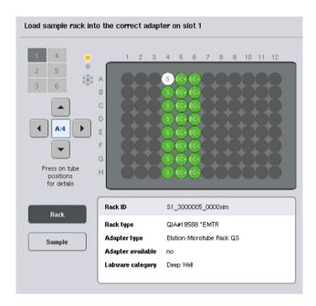
Press an individual position to view information about a particular sample. You can also use the arrows to select a position. When **Sample** is pressed, the sample ID, sample type, status, and sample volume are displayed, as well as the assay to which this sample has been assigned.
