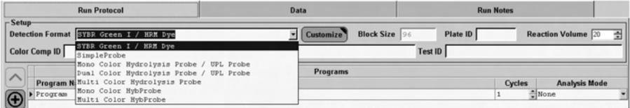
**Figure 8. Programming the LightCycler 480 for HRM analysis.** Choose detection format: SYBR Green I/HRM Dye. **Note:** If this channel for detection of EvaGreen dye is not chosen, reduced fluorescence may be observed.
