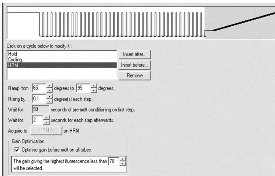
**Figure 7. Programming the Rotor-Gene system for HRM analysis.** Program the cycling protocol described in Figure 6 and Table 5. For HRM analysis, ramp from 65°C to 95°C, rising by 0.1°C each step.
