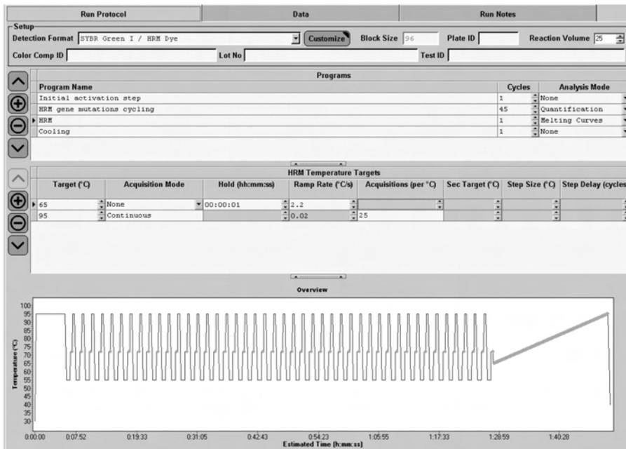
**Figure 5. Programming the LightCycler 480 system for HRM analysis.** Note: Times are entered in the format hh:mm:ss. Program the cycling protocol described in Figure 4. For HRM analysis, use 00:00:01 (1 s) at 65°C and 95°C. Select “Continuous” for “Acquisition Mode” with 25 acquisitions per second, resulting in a ramp rate of 0.02°C/s. Following HRM, samples should be cooled after the last cycle by entering 00:00:01 (1 s) at 40°C (not shown).
