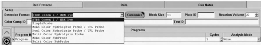
**Figure 3. Programming the LightCycler 480 for HRM analysis.** Choose detection format: SYBR Green I/HRM Dye. **Note:** If this channel for detection of EvaGreen dye is not chosen, reduced fluorescence may be observed.
