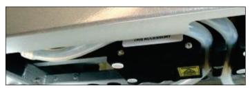
Hoses visible in the gap between the rear cover and the pinch valve.
