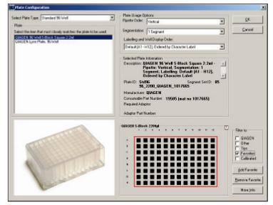
4. To display plates that are not tip racks, select QIAGEN and Other in the "Filter to" panel.
