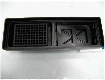
Channeling adapter and riser block EMTR inserted into the vacuum chamber.
