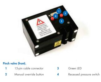
The pinch valve controls application of vacuum to separate vacuum chamber compartments for waste and elution during processing.
