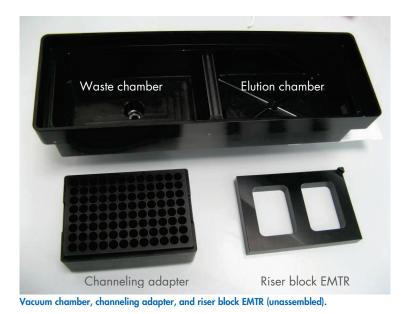
The QIAcube HT vacuum chamber is composed of two separate compartments for waste (left) and elution (right). This configuration is one of many measures that minimize sample cross-contamination during purification.
