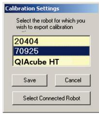
The "Calibration Settings" dialog box appears. Ensure that the displayed serial number matches the serial number of the connected instrument.
