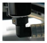
Each of these air bleeds has a small stainless steel aperture inserted in the hole to specifically control the rate of air flow.
