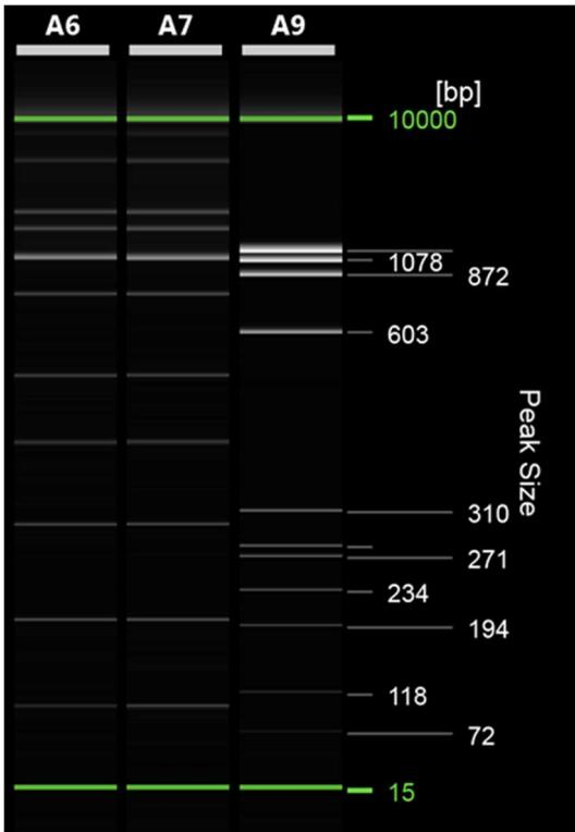
**Figure 8. Recovery of small DNA fragments.** A6: Ladder after purification using the 300  $\mu$ l protocol. A7: Equivalent amount before extraction. A9: QIAxcel DNA size standard.
