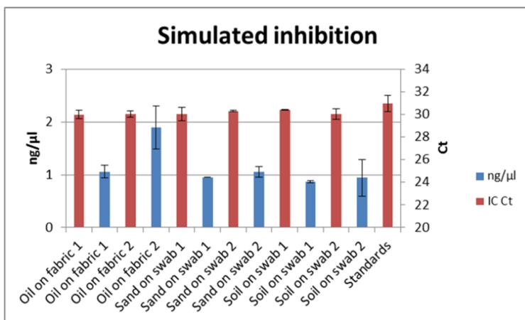
**Figure 5. Performance on inhibited samples for the 300  $\mu$ l protocol.** Blood from two donors (1 and 2) was used. Oil on fabric samples were processed in four replicates, swab samples in duplicates. DNA yield and the  $C_T$  values of the internal control (IC) of the Investigator Quantiplex HYres Kit are shown. The IC  $C_T$  values of the quantification standards serve as a non-inhibited reference.
