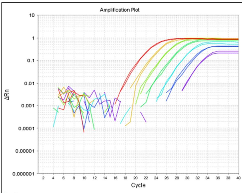
Figure 24. Example of an amplification plot for the human target of a standard curve for the Investigator Quantiplex HYres Kit.
