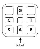
Schematic diagram of the PyroMark Q96 Cartridge (viewed from above). E: Enzyme Mixture; S: Substrate Mixture; G: dGTP; C: dCTP; T: dTTP; A: dATPαS.
