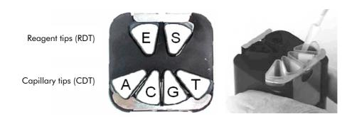
Arrangement of tips in the PyroMark Q96 Capillary Tip Holder. **E**: Enzyme Mixture; **S**: Substrate Mixture; **G**: dGTP; **C**: dCTP; **T**: dTTP; **A**: dATP $\alpha$ S.
