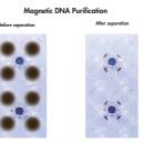
igure 1 Genomic DNA selectively binds to the surface of the MagAttract particles and an then be further purified by washing the magnetic particles. Magnetic rods, which it between the wells of a microplate or round-well block are used to attract all the particles o one side of the well, allowing the buffer to be removed
