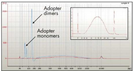
Figure 1. Precise size selection. The GeneRead Size Selection Kit effectively removes adapter dimers and adapter monomers following library preparation. A scaled-up image of the above data showing the correct size distribution of Illumina-compatible library fragments following size selection is shown in inset. FU: Fluorescence units.
