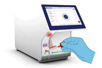
Figure 11. Scanning sample ID bar code.
