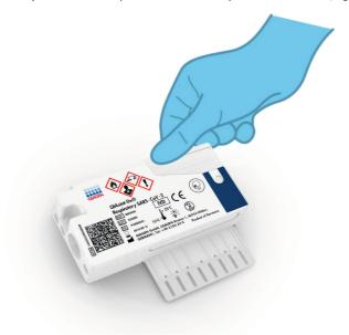
Figure 22. Closing the sample lid of the main port.
