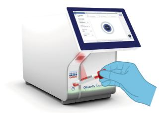
Figure 24. Scanning sample ID bar code.
