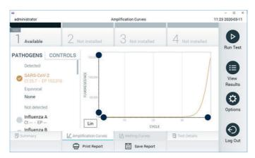
Figure 31. Amplification Curves screen (PATHOGENS tab).
