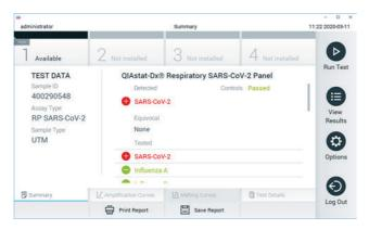
Figure 30. Results Summary screen example showing Test Data on the left panel and Test Summary in the main panel.
