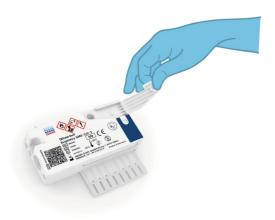
Figure 19. Opening the sample lid of main port.
