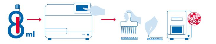
EZ2 Connect QIAcuity workflow. Up to 8 mL plasma can be processed on the EZ2 Connect combined with high eluate loading (up to 26 µL) on the QIAcuity.
