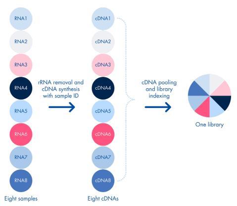
**Figure 3. QIAseq UPXome RNA Library Kit workflow.** Individual reverse transcription reactions are performed for each sample in the presence of a UPX barcoding oligo, which barcodes each cDNA. During a typical library preparation, up to 24 cDNAs are pooled together into a single library tube. The remaining reactions and library preparation steps associated with those 24 samples are performed in a single tube.
