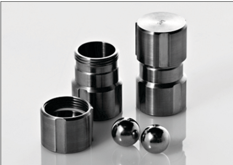
Figure 6. Grinding Jar Set, Stainless Steel. Each 10 ml jar is made of stainless steel and contains a 20 mm diameter stainless steel grinding ball.
