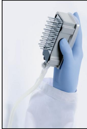
17. While holding the tool over the PyroMark Q24 Plate, close the vacuum switch on the tool (Off).
