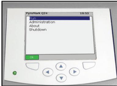
The instrument is controlled via the six buttons underneath the screen.
