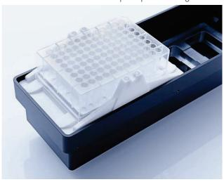
14. Gently twist the capture plate to secure it in the correct position.
