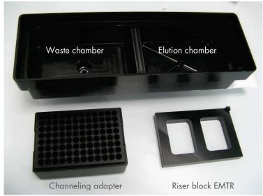
Vacuum chamber, channeling adapter, and riser block EMTR (unassembled).
