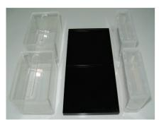
Reagent trough layout for the QIAcube HT specific reagent trough adapter.
