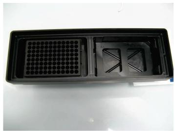
Channeling adapter and riser block EMTR inserted into the vacuum chamber.
