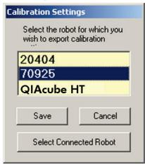
The "Calibration Settings" dialog box appears. Ensure that the displayed serial number matches the serial number of the connected instrument.
