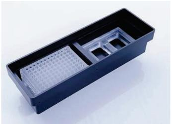
Waste sink/mat support and elution riser block inserted into the vacuum chamber.
