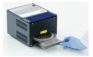
8. To activate the sealing mechanism, first press down on the blue anodized bar at the top of the Rotor-Disc Heat Sealer, and then push back the black catch.
