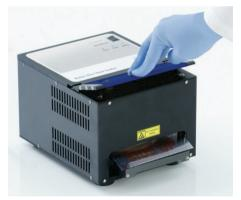
9. When sealing is finished, a long beep sounds and the orange "Ready" light starts blinking. Press down on the blue anodized bar to raise and lock the sealing mechanism back in its original position. Do not continue sealing for any longer than indicated by the beep or the Rotor-Disc may deform.
