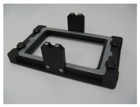
Transfer carriage for use with filter plates (e.g., QIAamp 96 plate)
