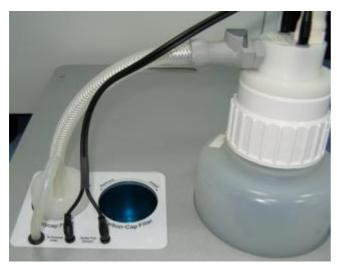
9. Plug the Carbon-Cap filter into the correct opening on the vacuum station. Be sure to position the filter with the labeling upside down.
