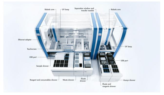
Figure 8. The QIAsymphony instrument with the SP and AS module.
