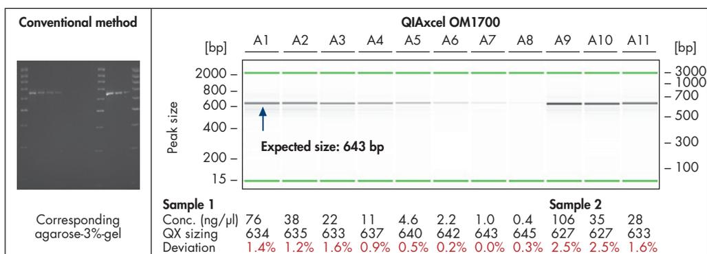
**Figure 1. QIAxcel Advanced performs accurate DNA fragment sizing.** Gel electrophoresis and fragment sizing of DNA fragments at various concentrations were performed using conventional gel electrophoresis and the QIAxcel Advanced instrument. Locus MIRU10 has repeats of 55 bp. The 643-bp fragment represents 3 alleles.
