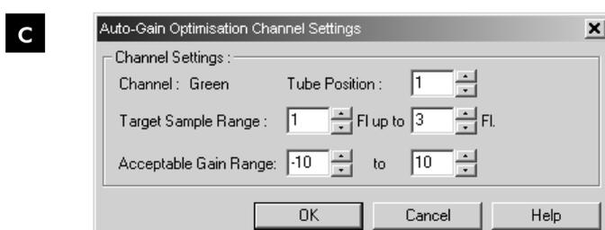
**Figure 4. Gain optimization for the Green channel.** **A** Select the Green channel, and click the “Gain Optimisation” button. **B** Click the “Optimise Acquiring” button. **C** In the pop-up box which appears, enter a “Target Sample Range” of 1 Fl up to 3 Fl. Then click “OK”, check the “Perform Optimisation Before 1st Acquisition” box, and click “Close”.
