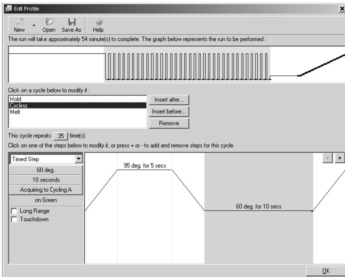
**Figure 2. Two-step cycling.** PCR requires 35 cycles. Each cycle is comprised of 2 steps: 95°C for 5 s (denaturation step) and 60°C for 10 s (annealing/extension step).
