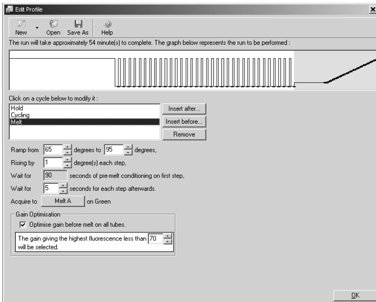
**Figure 3. Melting curve analysis.** After PCR is completed, melting curve analysis can be performed to check the specificity of the reaction. Ensure that the “Optimise gain before melt on all tubes” check box is checked.
