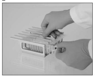
Figure 3. Ease of instrument setup using reagent cartridges (RCV). A A sealed, prefilled reagent cartridge (RCV). Fill levels vary, depending on the type of reagent cartridge (RCV). Loading reagent cartridges (RCV) into the cartridge rack. The cartridge rack itself is labeled with an arrow to indicate the direction in which reagent cartridges (RCV) must be loaded.
