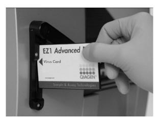
**Figure 1. Ease of protocol setup using EZ1 DSP Cards.** Inserting an EZ1 Card, preprogrammed with the protocol, into the EZ1 instrument.
