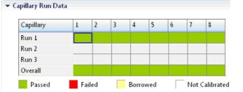
Figure 3. Example of successful spectral calibration of the Matrix Standard BT6 for all capillaries on an Applied Biosystems 3500 Genetic Analyzer.
