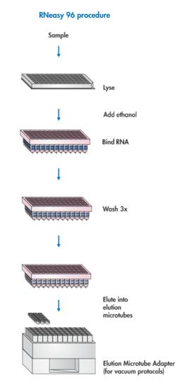
Figure 1. RNA isolation with the RNeasy 96 Kit. Protocol steps can be performed on a QIAvac 96 vacuum manifold (with the Elution Microtube Adapter shown) or in a specially designed centrifuge system (see page 11).
