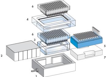
Figure 2. Components of the QIAvac 96 vacuum manifold
