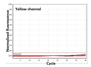
**Figure 8. The PCR is inhibited**. No amplification of the three samples in the green channel (left) or the internal control in the yellow channel (right). All curves lie along the baseline and do not exceed a preset threshold.
