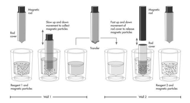
**Figure 2. Schematic of the QIAsymphony SP principle**. The QIAsymphony SP processes a sample containing magnetic particles as follows. A magnetic rod protected by a rod cover enters a well containing the sample and attracts the magnetic particles. The magnetic rod cover is positioned above another well and the magnetic particles are released. The QIAsymphony SP uses a magnetic head containing an array of 24 magnetic rods, and can therefore process up to 24 samples simultaneously.
