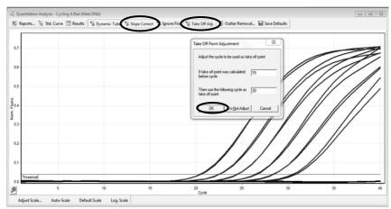
Slope correction and Take Off Point Adjustment tool.
