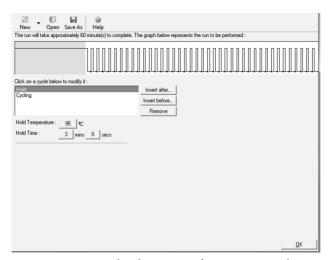
Initial PCR activation step. PCR requires an initial incubation at 95°C for 3 min to activate the DNA polymerase.
