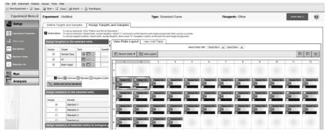
Setting up the standard curve and assigning the samples to the plate layout.
