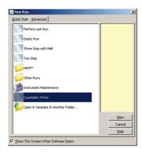
10.To setup cycling manually, select "Two Step" cycling profile, and click "New."
