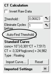
Setting the C<sub>T</sub> value for the Green Channel using the Auto-Find Threshold.
