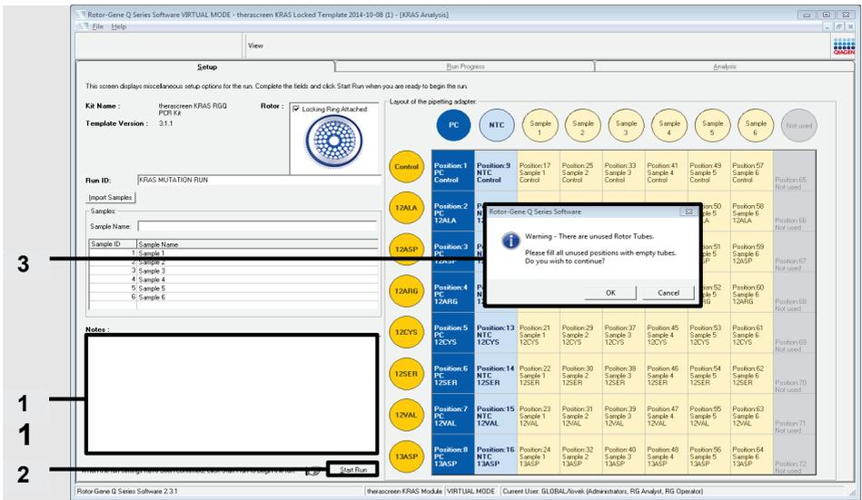
**Note:** If any rotor position is unused, a warning will appear (3 above and 1 in example below) to remind the user that all unused positions on the rotor must be filled with a capped, empty tube.
