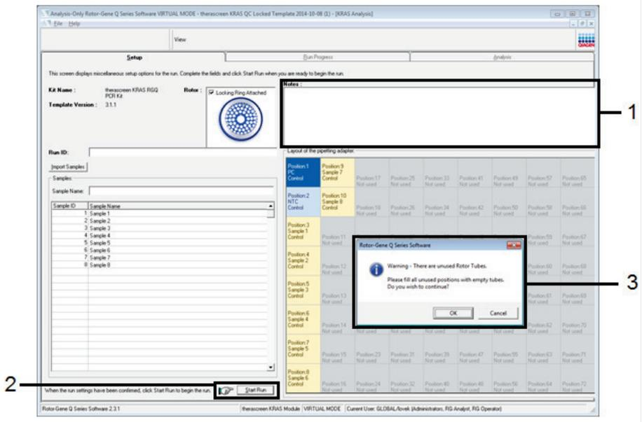
**Note:** If any rotor position is unused, a warning will appear (3 and example below) to remind the user that all unused positions on the rotor must be filled with a capped, empty tube. Check that all unused rotor positions are filled with a capped, empty tube and click **OK** (1 in the example below) to proceed.
