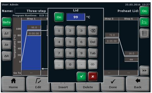
Figure 20. QIAamplifier 96 heated lid temperature setting screen.
