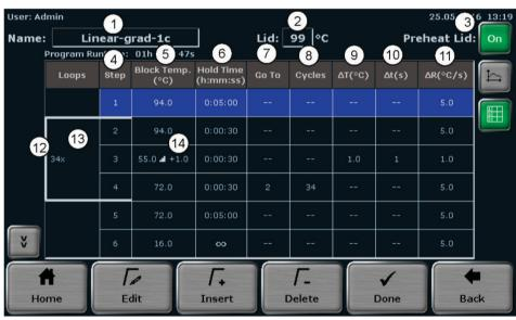
Figure 15. Spreadsheet programming.
