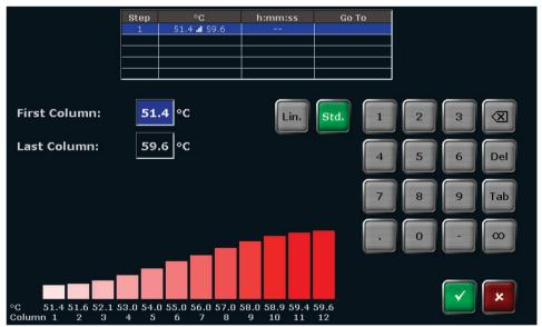
Figure 24. QIAamplifier 96 standard gradient programming screen.
