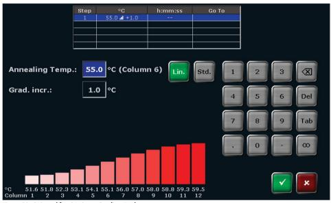
Figure 23. QIAamplifier 96 Linear Gradient Tool screen.
