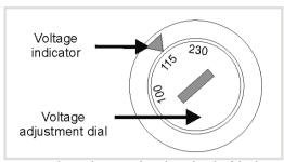
Figure 2. Voltage selector switch on the underside of the device.
