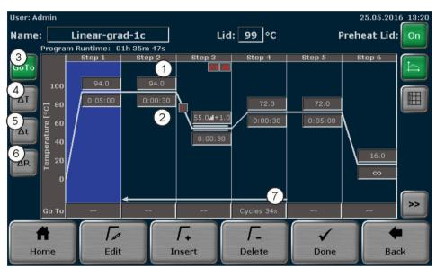
Figure 26. QIAamplifier 96 graphical program view.
