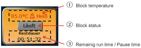
Figure 12. QIAamplifier 96 block status/quick start button.
