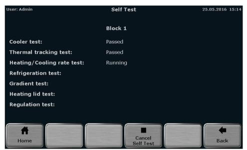
Figure 62. QIAamplifier 96 extended self-test overview screen.
