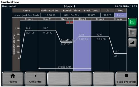
Figure 38. QIAamplifier 96 run display screen during a program pause.
