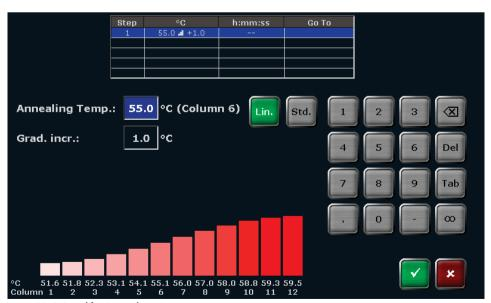
Figure 28. QIAamplifier 96 gradient view.
