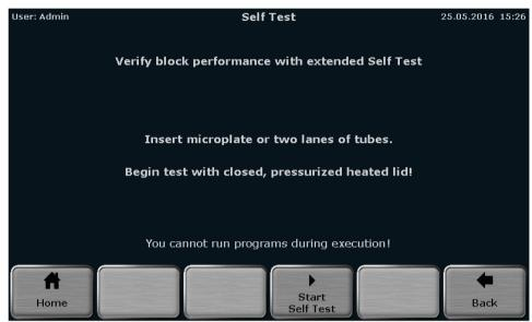
Figure 61. QIAamplifier 96 extended self-test screen.
