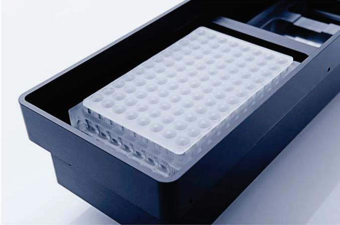
11. Check of the sealing lip of the capture plate to be sure there are no chips or cracks.
