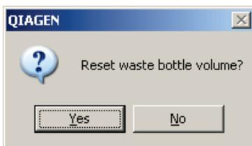
When the bottle fills with 3 liters of waste, the liquid comes into contact simultaneously with 2 Teflon<sup>®</sup> coated sensor electrodes within the waste bottle. When this occurs, the software pauses the run until the waste bottle is emptied and the waste indicator is reset.
