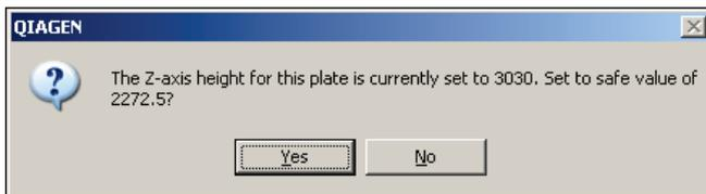
If the current setting is retained and the plate in the position is too high, the tip may jam into the plate and bend.
