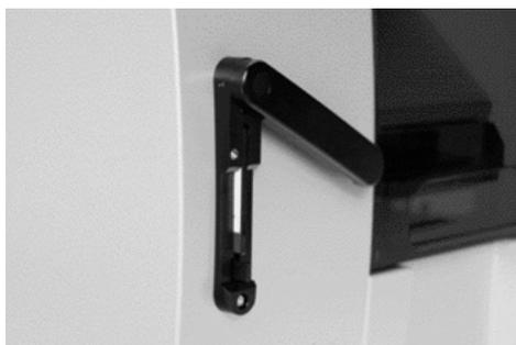
**Figure 3. EZ1 Card completely inserted into EZ1 Card slot.**
