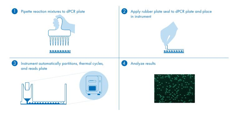
Figure 5. Setup of dPCR reactions. Four simple steps from sample to insight.
