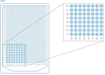
Figure 3. Representation of the two different 384 MTP layouts set in the cellenONE X1 for cell isolation. A 384 MTP layout for isolation of one single cell per well. B 384 MTP layout for isolation of different numbers of cells per well.
