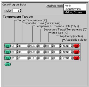
5. Select "None" and set up the parameters for cooling as shown below.
