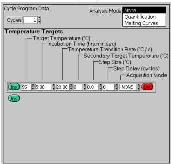
3. Select "Quantification" and set up the parameters for PCR cycling as shown below. Be sure to select "SINGLE" for "Acquisition Mode" at the 60°C step.
