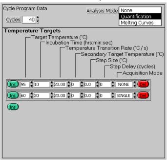
4. Select "Melting Curves" and set up the parameters for melting curve analysis as shown below. Be sure to select "CONT" for "Acquisition Mode" at the 95°C step.
