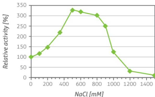
**Fig. 3.** The effect of  $\text{Na}^+$  ions on the Saltonase activity.
