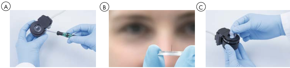
Figure 12. Replace release needle. A. Loosen the screws from the release device using the screw driver. B. Handle the replacement window containing the needle by the edges. C. Gently place the replacement window containing the needle on the release device.
