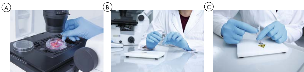
Figure 11. Transfer of released microraft. A. Bring the magnetic wand close to the released microraft. B. Depending on your downstream experiment, place the wand in a suitable reaction tube (here a 1.5 ml reaction tube) or any other secondary vessel of your choice. C. Place the tube, in which the magnetic wand is still inserted, onto the center of the magnetic collection plate and hold firmly.
