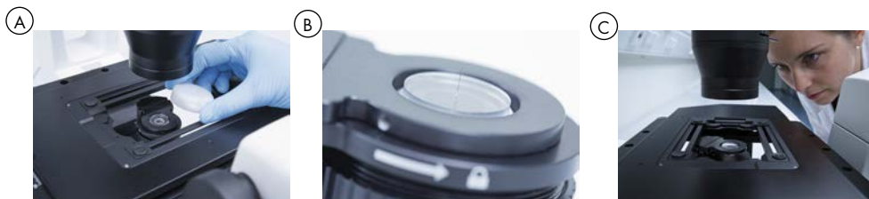
Figure 5. Release device installation. A. Carefully remove the protective lid. B. The needle is delicate, do not touch or bend it. C. Ensure there is no collision of the release device with other microscope parts.
