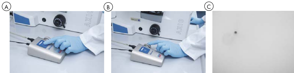
Figure 7. Calibration of the QIAscout instrument. A. Long (2 s) press the button to set up calibration mode. B. Turn the wheel to adjust release needle height. C. Turn the wheel up until the small bright dot (indicative of the tip of the release needle) is visible.
