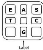
**Figure 1. Illustration of the PyroMark Q24 Cartridge as seen from above.** The annotations correspond to the label on the reagent vials. Add Enzyme Mixture (E), Substrate Mixture (S) and nucleotides (A, T, C, G) according to the volume information given in the **Pre Run Information** report, found in the **Tools** menu at run setup.
