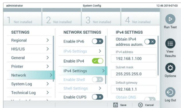
Figure 1. Configuring a static IP Address on the QIAstat-Dx Operational Module.
