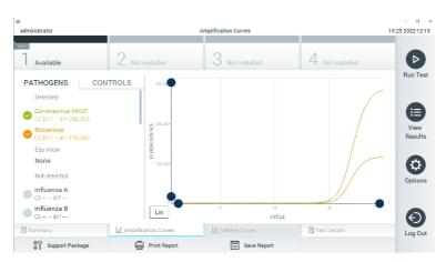
Figure 32. Amplification Curves screen (PATHOGENS tab).
