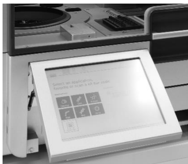
Figura 16: Ecranul tactil extras al QIAcube Connect MDx.
