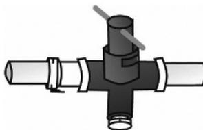
Figure 3. Main vacuum valve in the closed and open position.
