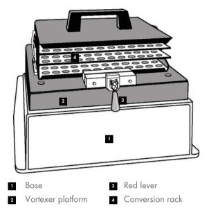
All of the operating controls for the MST Vortexer 2 are located on the front panel. The following figure shows the front panel.
