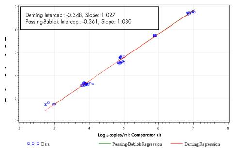
Figure 3. Regression plot with Passing-Bablok and Deming Lines for CSF samples. Samples that are between the lower limit of quantification and the upper limit of quantification for both kits were included in the analysis.
