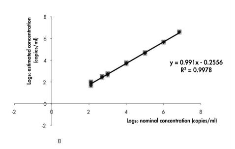
Figure 6. Linear range of the artus VZV QS-RGQ Kit (plasma). Calculation of the linear range. The straight line was determined by a linear regression of the log<sub>10</sub> calculated concentrations with the log<sub>10</sub> nominal concentrations. The equation of the regression line is included in the figure.
