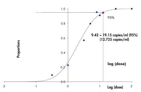
Figure 5. Probit analysis: plasma, VZV (Rotor-Gene Q). Analytical sensitivity in consideration of the purification (using the QIAsymphony DSP Virus/Pathogen Midi Kit) and the artus VZV QS-RGQ Kit on the Rotor-Gene Q.
