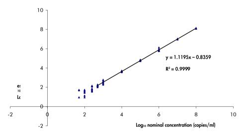
Figure 2. Linear range of the artus VZV QS-RGQ Kit (CSF). Calculation of the linear range. The straight line was determined by a linear regression of the log<sub>10</sub> calculated concentrations with the log<sub>10</sub> nominal concentrations. The equation of the regression line is included in the figure.
