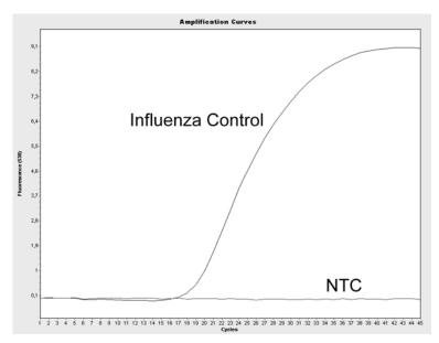
**Figure 17. Detection of the Influenza Control in channel F1.** On the LightCycler 2.0 instrument, the Influenza Control is detected in fluorescence channel 530. **NTC**: No template control (negative control).
