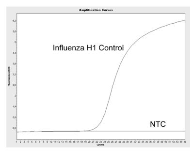
**Figure 19. Detection of the Influenza H1 Control in channel F1.** On the LightCycler 2.0 instrument, the Influenza H1 Control is detected in fluorescence channel 530. **NTC**: No template control (negative control).
