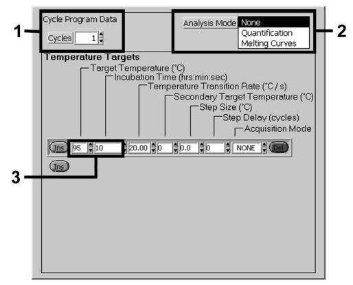
Figure 14. Initial activation of the hot-start enzyme.
