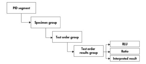
If preliminary results are included, the derived result is sent first. Following the derived result, the constituent measurement records are sent.
