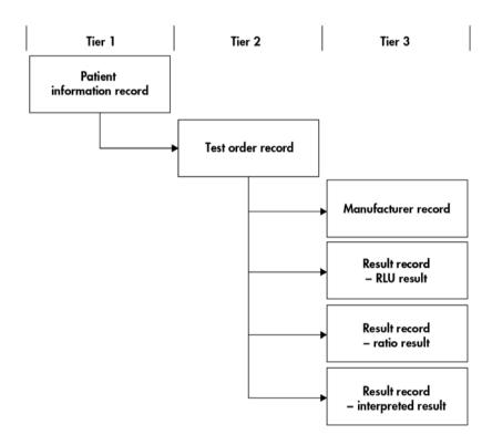
If preliminary results are included, the test order and result records are sent twice. The derived result, containing a test order and a result record for the interpreted result, is sent first. Following the derived result, the constituent measurement records, containing the test order record, result record for the RLU result, result record for the ratio result and the result record for the interpreted result, are sent.
