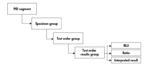
If preliminary results are included, the records are transmitted for each constituent test performed. The maximum number of constituent tests, as defined by the retest algorithm, is three. The following minimum records are exported for each specimen:
