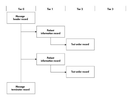
Test orders are rejected at the patient information record level. If two test order records are associated with the same patient information record and one test order record contains an error, both test order records will be rejected.
