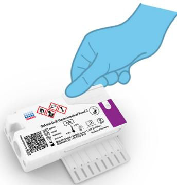
**Figure 8. Closing the lid of the main port.**
