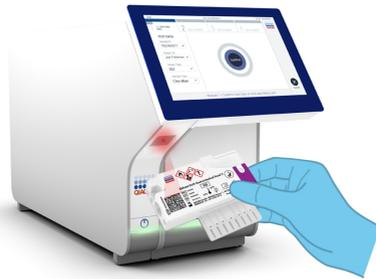
**Figure 11. Scanning QIAstat-Dx Gastrointestinal Panel 2 Cartridge bar code.**
