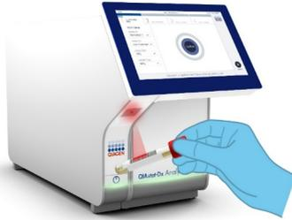
**Figure 10. Scanning sample ID bar code.**
