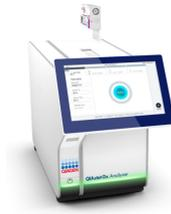
**Figure 13. Inserting QIAstat-Dx Gastrointestinal Panel 2 Cartridge into QIAstat-Dx Analyzer 1.0 or the QIAstat-Dx Analyzer 2.0.**
