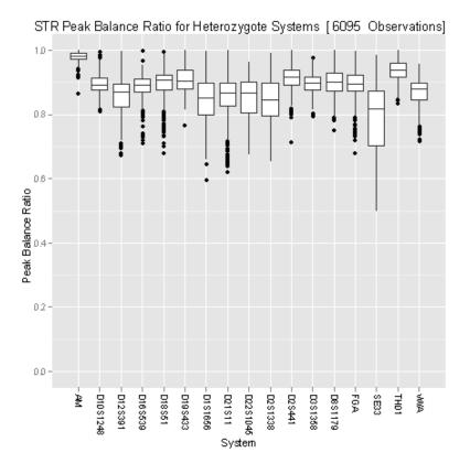
**Figure 18. Box plot analysis of intra-locus peak height ratios.** Values refer to the lower of the 2 peaks in a heterozygous sample. Boxes represent the middle 50% (interquartile range, [IQR]) of data, and lines inside the boxes represent the median. Whiskers show data within 1.5 IQR, and dots represent outliers.
