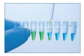
Figure 2. Accurate reaction setup indicated by the built-in pipetting control. The QuantiNova SYBR Green PCR Master Mix contains an inert blue dye. Combined with QuantiNova Yellow Template Dilution Buffer, the resulting solution turns green, indicating that the reaction was set up correctly.
