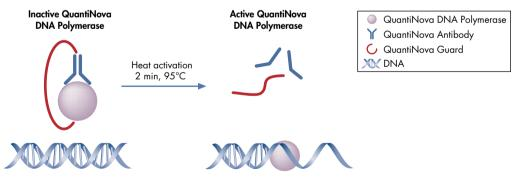
Figure 1. Mechanism of the highly stringent QuantiNova hot-start. Sequestered in a binding complex with the QuantiNova Antibody, QuantiNova DNA Polymerase is kept in an inactive state until the initial heat activation step denatures the complexstabilizer QuantiNova Guard and the QuantiNova Antibody.
