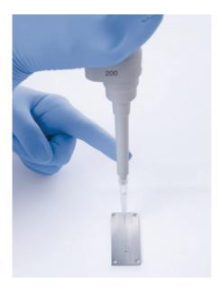
Figure 2. Correct dispensing technique for transferring beads to the flow cell port.
